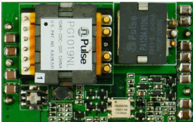
FIGURE 1. TOP VIEW OF ISL6726EVAL1Z (ACTUAL SIZE: 40x60x16mm)
